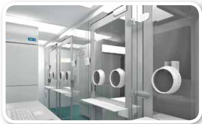
Four (4) Infectious Disease Diagnostic Sampling Booth™ (IDDSB™) units in 20ft containers equipped with a fully integrated BSL laboratory inside for swabbing and storage of diagnostic samples.
